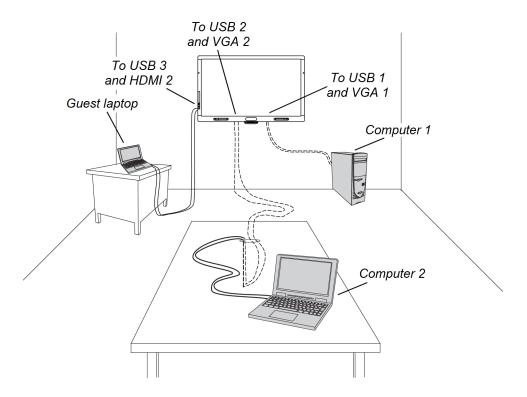
Connect video cables to the bottom terminal panel and connect USB cables to the inside terminal panel.
