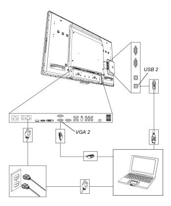
You require a USB cable and a VGA cable to set up the computer 2 connection location.
