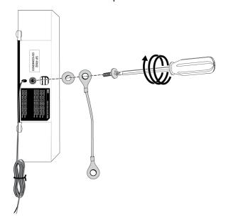
2. Above the speaker mounting holes, remove the screw and washer.
