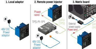
TPS-TX/RX90 and TPS-TX/RX95 are not PoE-compatible, thus not able to remote power the WP-HDMI-TPS-TX/97 series and vica versa. WP-UMX-TPS-TX97 series contains PoEcompatible remote power function (PD. Powered Device). RX95 and TX95 extenders can be remote powered only by each other.
