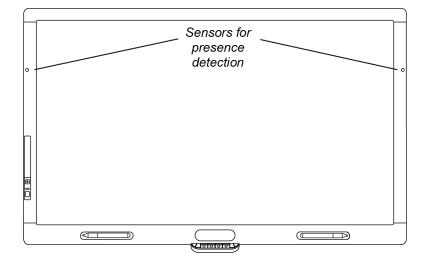
The interactive flat panel has two presence detection sensors on its frame that can detect people up to 16' (5 m) away when the interactive flat panel is in Standby mode.
